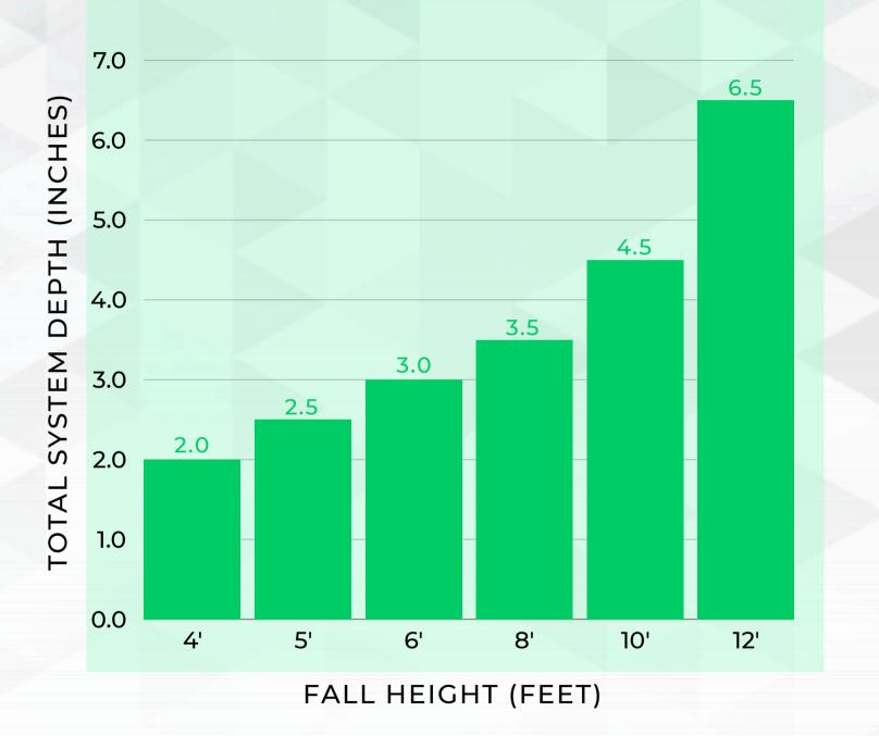
CHART REPRESENTS THE TOTAL (SBR CUSHION & TPV WEAR COURSE) SYSTEM DEPTH EXAMPLE: 2.5" SYSTEM CONSISTS OF 2" SBR CUSHION LAYER AND APPROX. 1" TURF WITH .5" INFILL
